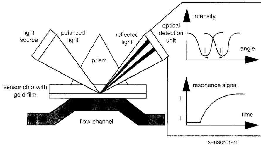
**FIGURE 18-22 Schematic of SPR**
