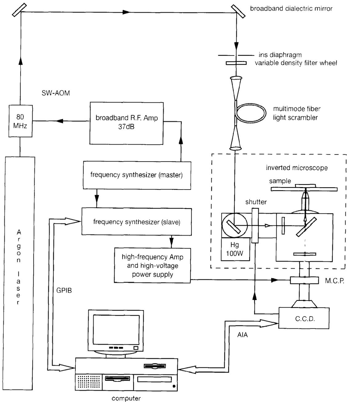
**FIGURE 18-18** Schematic of a Single-frequency FLIM Configuration
