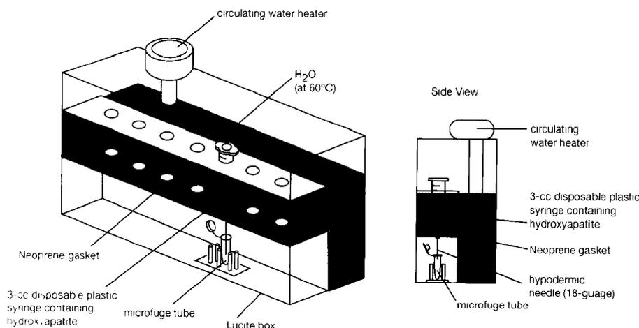
**FIGURE A8-4** Apparatus for Hydroxyapatite Chromatography
