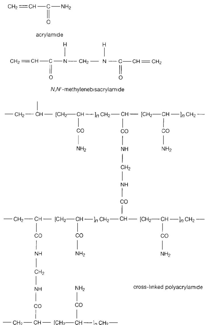
**FIGURE 5-6 Structure of Polyacrylamide**
