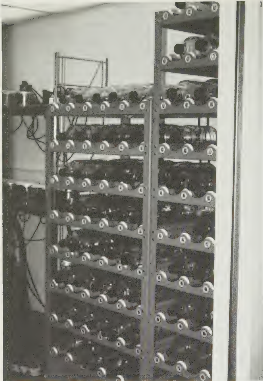
FIGURE 1. Photograph of roller bottle deck assembly.
