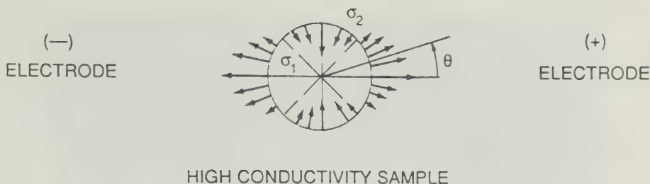
FIGURE 7. Cross-sectional diagram of high conductivity sample showing surface stress vectors acting on a cylindrical sample stream with long axis perpendicular to the electric field.
